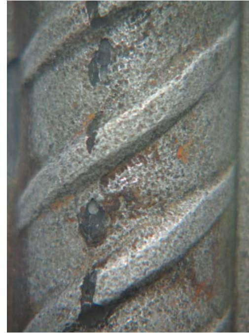
Sandblasted 3Cr12: extensive corrosion, pits and general
