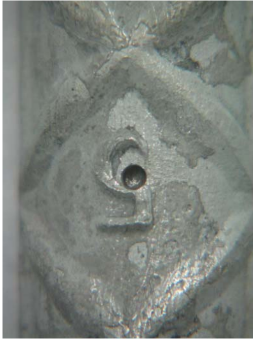
Galvanized-type A: extensive corrosion, many parts lost Zn coating. Steel in hole was largely protected
