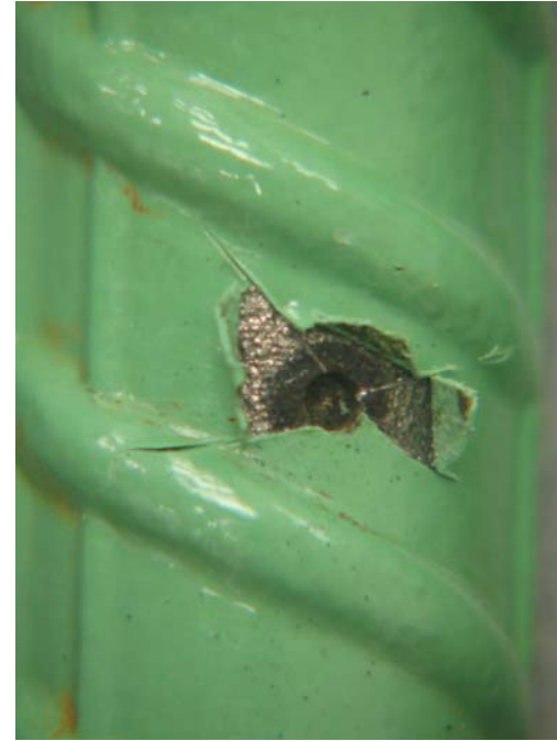
ECR-Type A- adhesion: dark area lost adhesion, rate- 2.5
