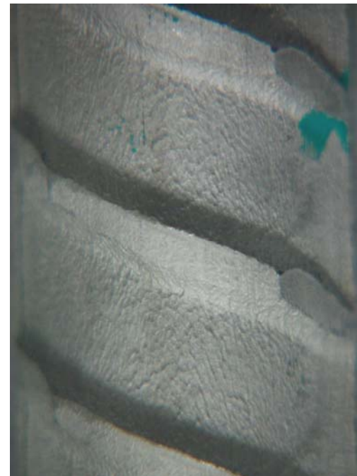
As received 316LN: pristine condition except minor corrosion at bar ends
