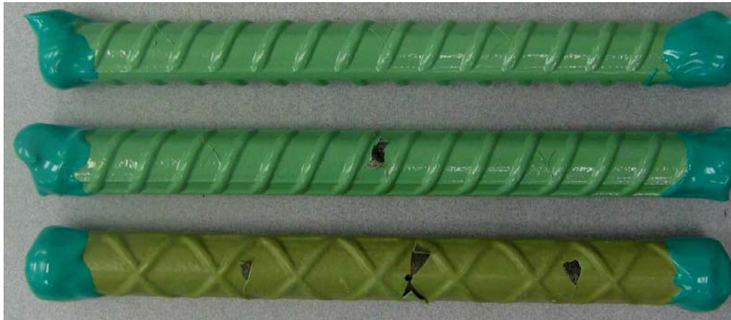
Figure 9. Knife adhesion test of Epoxy-coated bars after 4 weeks of exposure. From top to bottom: ECR-Type A-no hole; ECR-Type A-hole; ECR-Type B-hole
