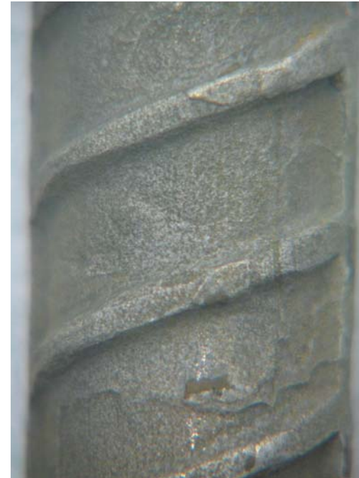
Sandblasted A615 bar: extensive corrosion, more uniform
