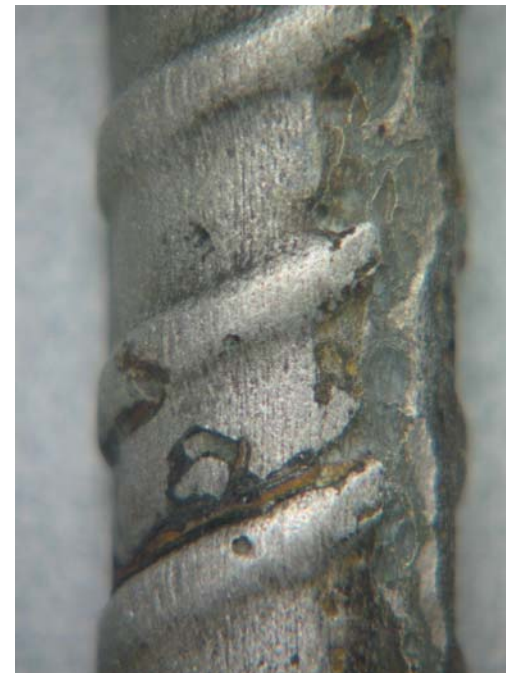
Sandblasted A1035: broader pitting attack
